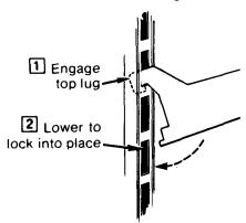
To replace shelves: Select desired shelf height. With shelf front raised slightly, engage top lugs in tracks at rear of cabinet. Then lower front of shelf until it locks into position.
